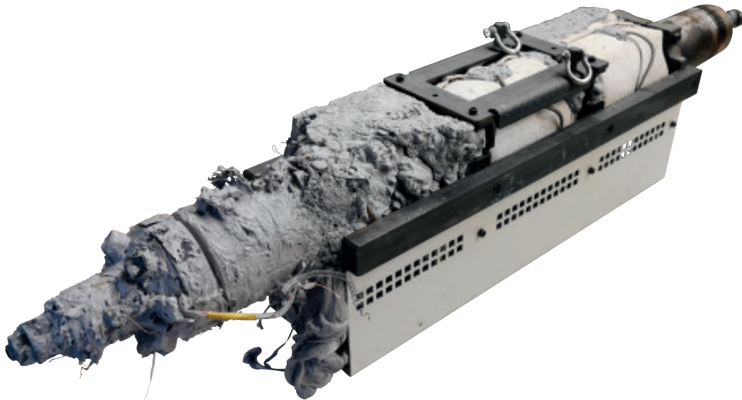
plastification unit before repair
